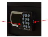
USB (ONLY USED TO CONNECT THE OPTIONAL HANDHELD ELECTRONIC DEVICE C.E.U.70)
