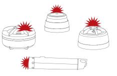
6. When all alarms flash the red LED, they are connected and can be switched out of "Learn mode" and installed.
